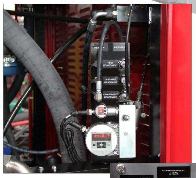
For those who want to document test component cleanliness on test reports and want real time feedback on the cleanliness of their Hydraulic Test Center (HTC). The Contamination Monitoring accessory eliminates the delay of bottle sampling. The Contamination Monitoring accessory fully integrates into the HTC and offers real-time cleanliness level measurement
